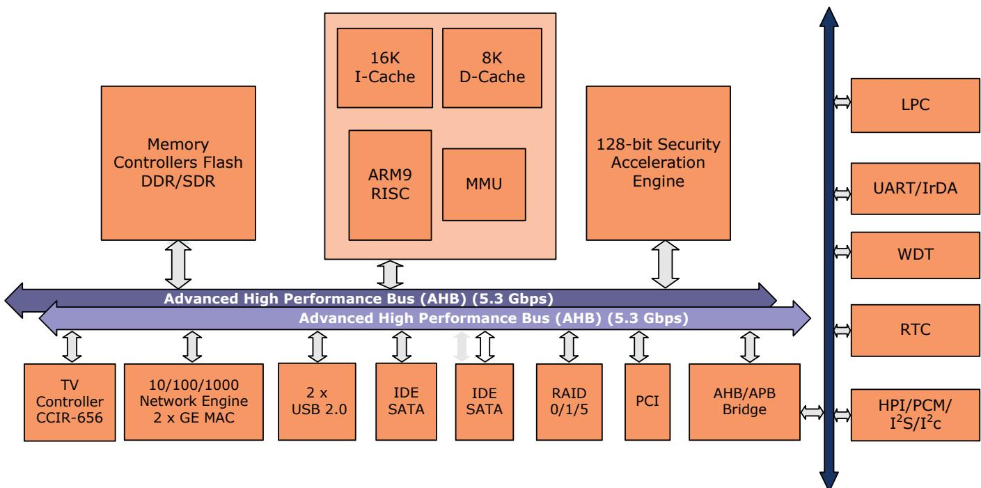
CS3516 Network Processor Block Diagram
